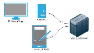
Figure 6.3 Deployment architecture diagram
